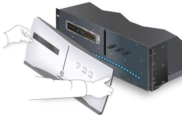
Figure 2 Removing the Front Panel
