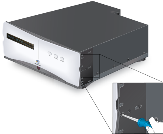
Figure 1 Removing Rack Ears
