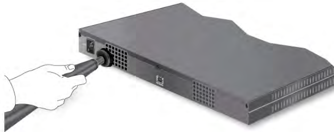
Figure 16 Vacuuming Reader Rear Outlet Grilles
