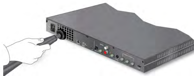
Figure 13 Vacuuming Movie Player Rear Outlet Grille
