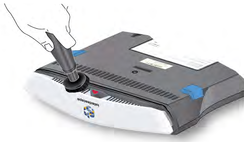
Figure 9 Vacuuming M300 Player Air Inlet Grilles
