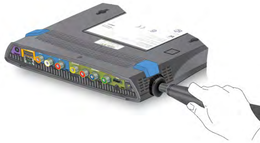
Figure 11 Vacuuming M300 Player Side Grilles
