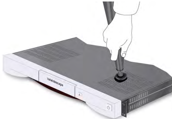
Figure 15 Vacuuming Reader Top Grilles
