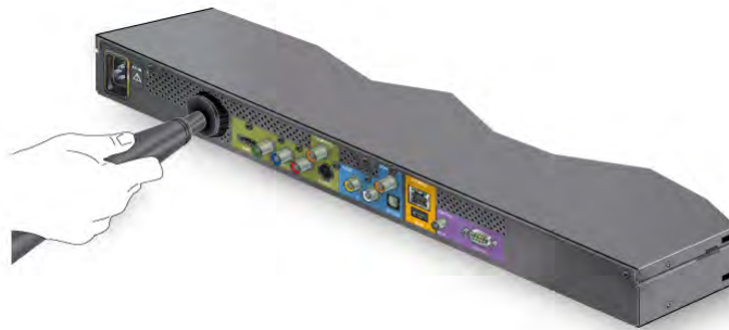
Figure 5 Vacuuming M500 Player Air Outlet Area
