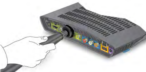
Figure 10 Vacuuming M300 Player Air Outlet Grille
