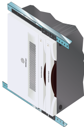
Figure 3 Vertical Mounting of 5U Server with Movie Players
